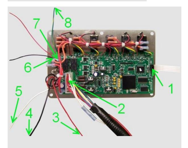
Numbers 1, 2, 6, and 7 must be disconnected from the control board.
